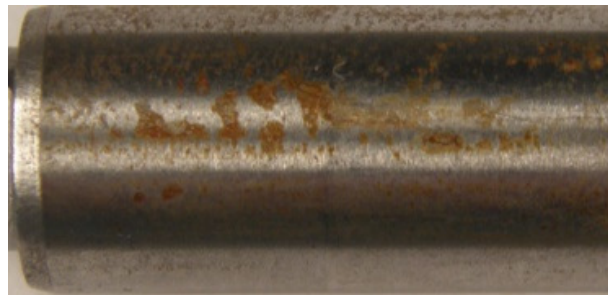
Fig. 2. Corrosion on shaft throttle
